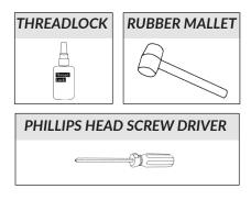
We strongly recommend assembling on a flat surface, applying thread lock to the full length of all screws and using a screwdriver.
